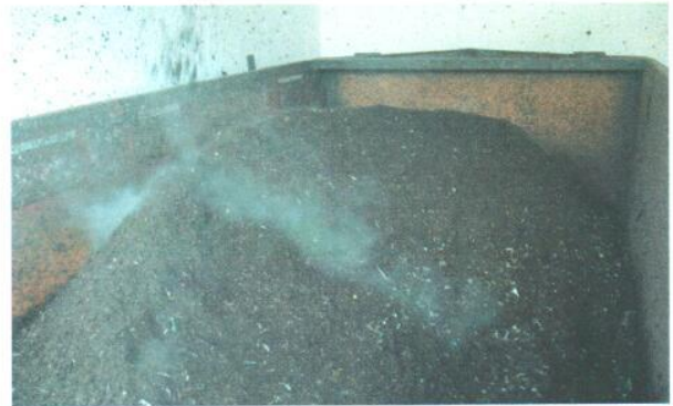
Output from anaerobic digestion
